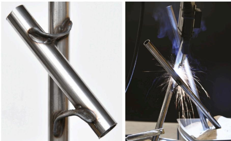
Fig. 9. Ariza et al. 2018 [41] developed adaptive in-place detailing methods through WAAM for joining steel members.
