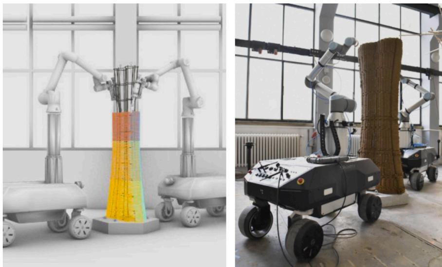
Fig. 16. Cutajar et al. 2024 [81] show a homogeneous dual-robot setup utilised to 3DP an earthen formwork for concrete casting cooperatively from opposite sides with finger joints in between the meeting points of the segments.
