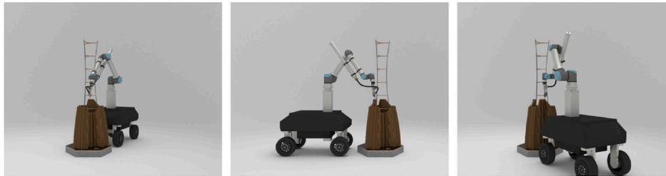
**Fig. 11.** In Dielemans et al. 2020 [18], segments (here: segments 19, 20, and 21) of a larger structure are manufactured within the static reach of the mobile robot, allowing for sequential navigation and manipulation. Optimal task segmentation considers the workspace limitations of the respective robot in use.
