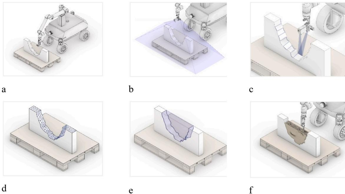
**Fig. 4.** Proposed workflow and stepwise method for in situ repair of an incomplete wall geometry: a) mobile robot positioning & object framing, b) initial 3D point cloud capture, c) refined 3D point cloud capture, d) reconstructed surface, e) repair design, and f) repair design & print path generation, by Dielemans et al. 2024 [23].
