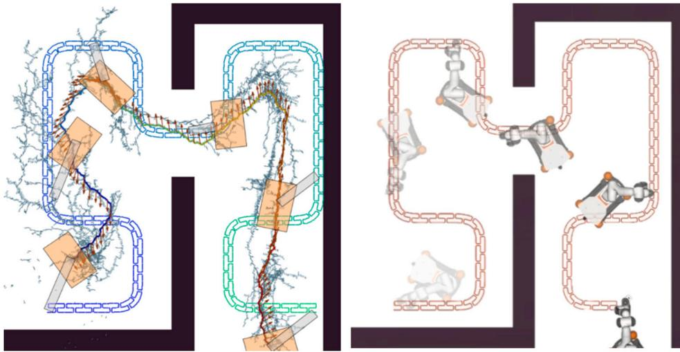
**Fig. 13.** A path planning illustration. Static Obstacles (Black), Print Task (Blue to Green), b(s) found (Blue to Red), RRT\* tree exploration, visible in blue, shown only in 2D, for 3DP in motion, as shown in Sustarevas et al. 2021 [47].
