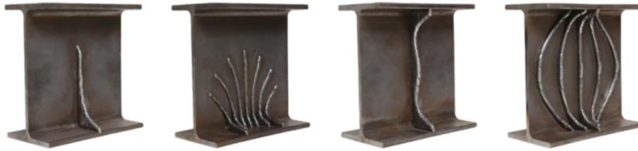
Fig. 8. WAAM stiffeners on IPE200 profiles, introduced by Kloft et al. 2023 [40]
