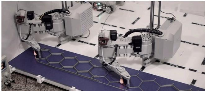
**Fig. 12.** With the Ambots project, generating viable print schedules with collision-free path planning allows multiple robots to cooperate on a single 3DP job. AMBots Inc. 2020, Video frame from [89]
