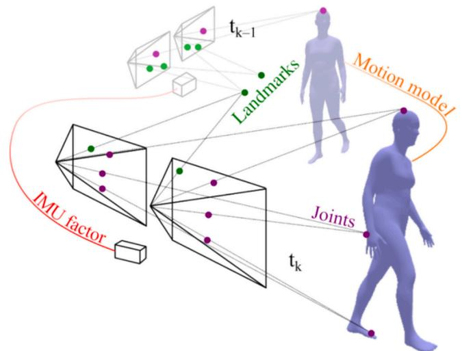
**Fig. 14.** The BodySLAM++ framework by Henning et al. [62] uses an IMU factor between frames and a human motion model to predict the displacement of the sensor and human, respectively, making it particularly apt to be integrated into mobile construction robots.
