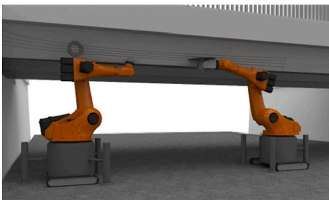
**Fig. 17.** Vision for a heterogeneous dual-robot setup aimed at strengthening structural components, including milling channels for reinforcement, and forming the bond between reinforcement and concrete through concrete 3DP. Source: D. Lowke
