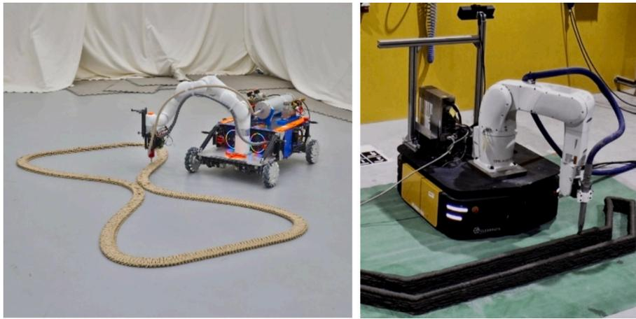
Fig. 1. Examples of mobile manipulators (left: Sustarevas et al. 2022 [19], right: Tiryaki et al. 2019 [17]) carrying out mobile extrusion 3DP tasks in full motion, that is, in printing-while-driving fashion.
