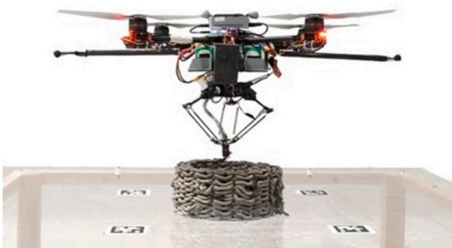
Fig. 2. Aerial Additive Building Manufacturing, published by Zhang et al. in 2022 [22], has showcased the potential of using drones for M3DCP tasks for building construction and repair.
