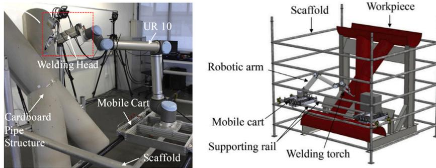
**Fig. 10.** The robotic system and the lab experimental setup introduced by Dharmawan et al. [43] and Chen et al. [88] consists of a representative dummy weld head equipped with a 2D laser scanner and a 1:1 scale mock-up jackup rig pipe structure.
