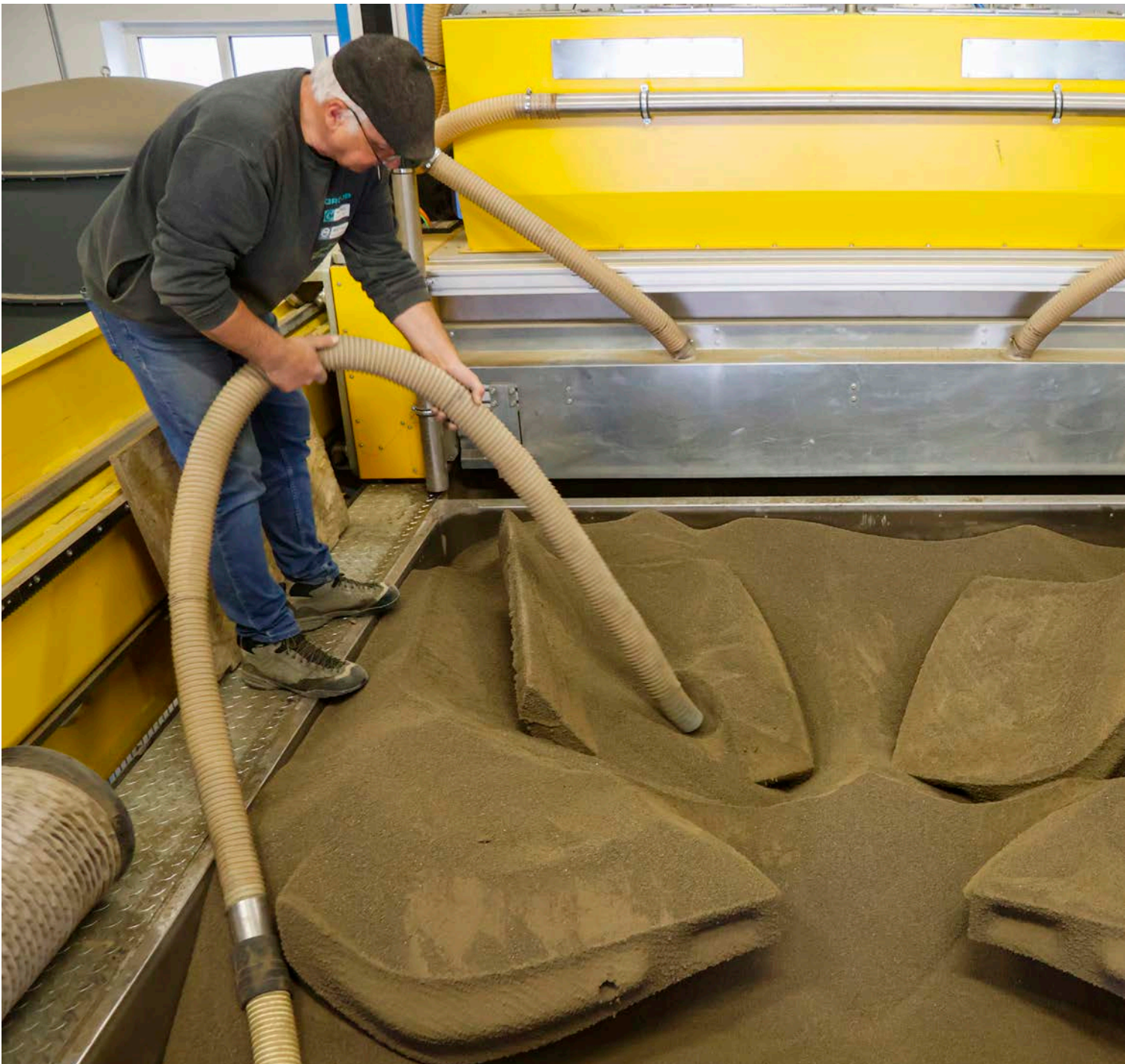
SPI method utilised for closed-cell geometries with trapped lightweight aggregates: a) deposition of aggregate layer; b) selective binding with a cement-paste, c) excavated component. © Krakovská et al. 2024
