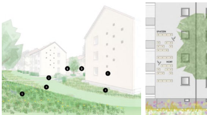
Figure 4: Integration of nests into buildings' facades, Weisser & Hauck Fundamentals
