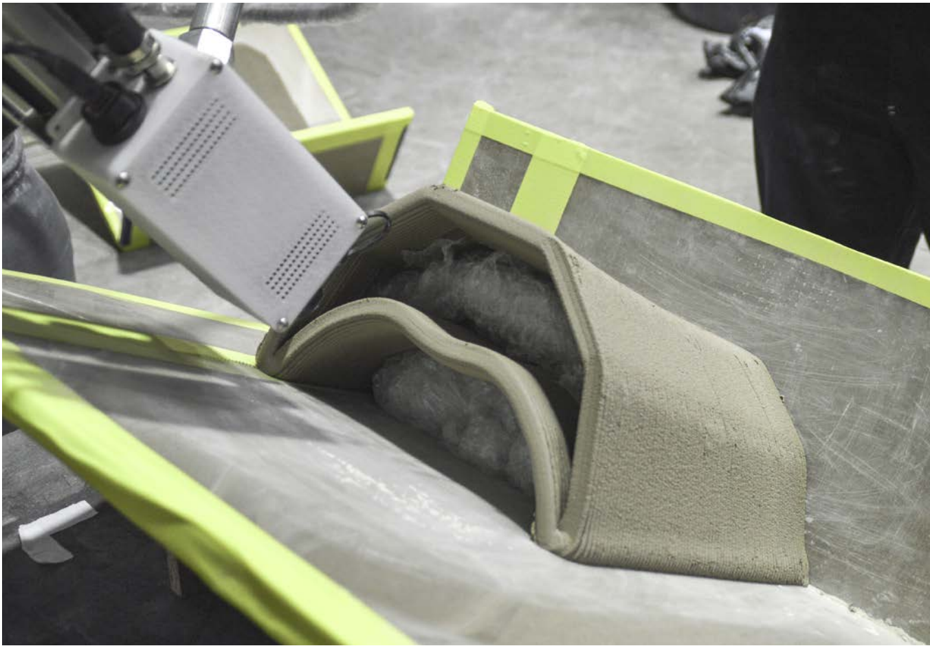
Printing with substructure 30 degree | Nest element
