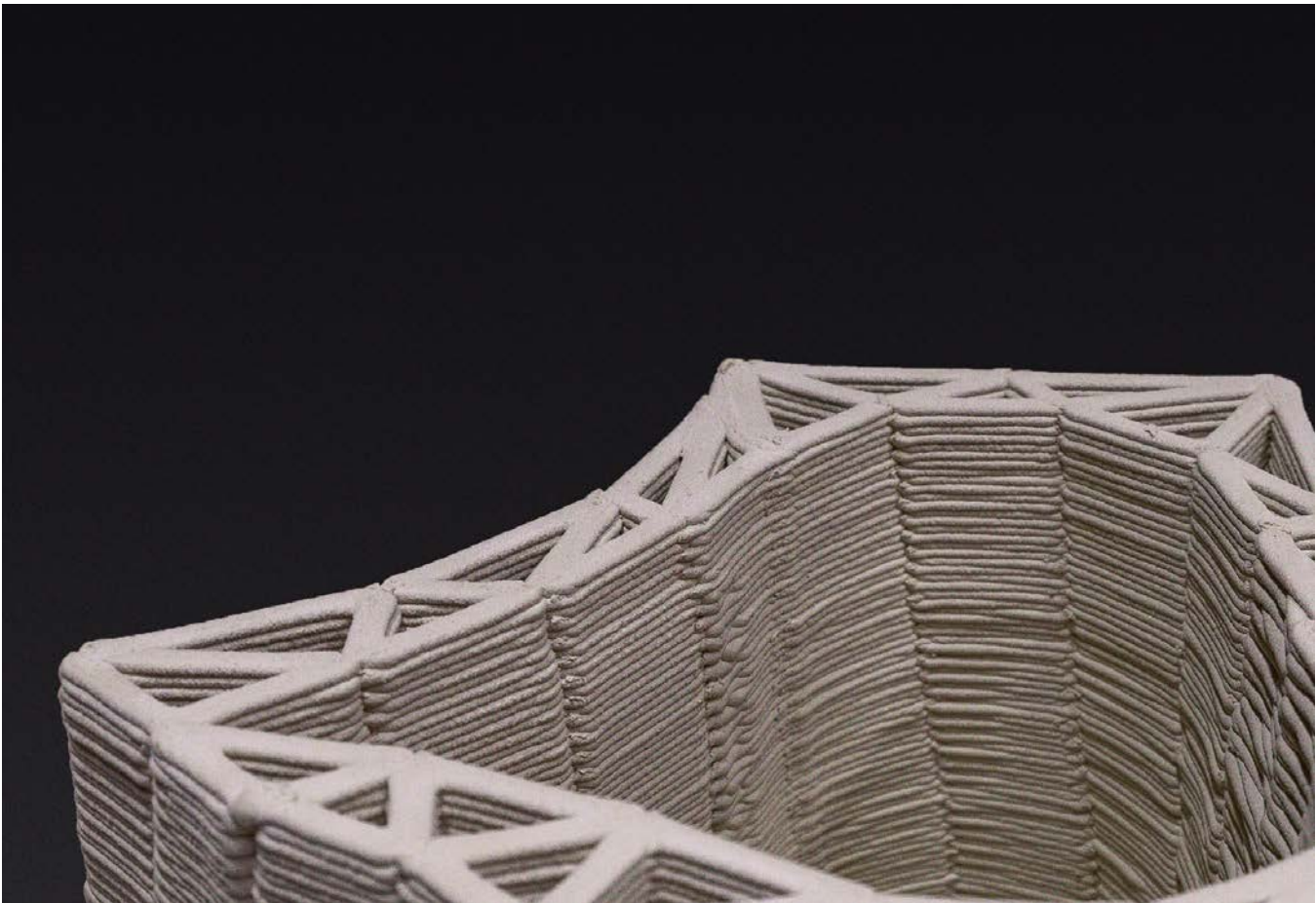
Detail of support structure which simultaneously forms inner and outer shell.
