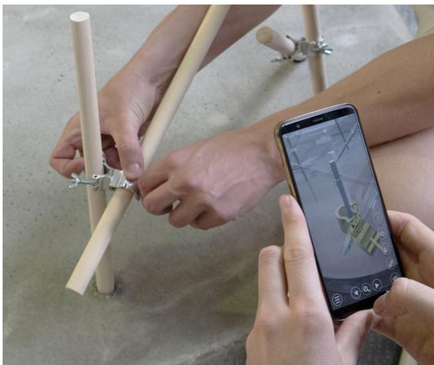
**Fig. 6** Connecting two elements with the zoom in feature of the AR application
