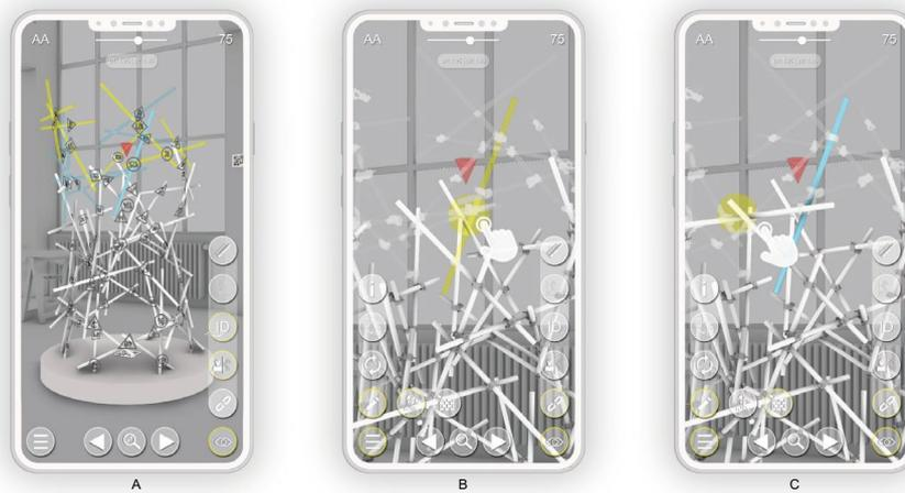
**Fig. 9** (A) Visualizing the index and type of each unbuilt element, along with the assigned executor for its placement, (B) Adjusting the executor of an element by enabling the “Parameter Adaptation Menu” and selecting the preferred element, (C) Modifying the “Built Status” of an element
