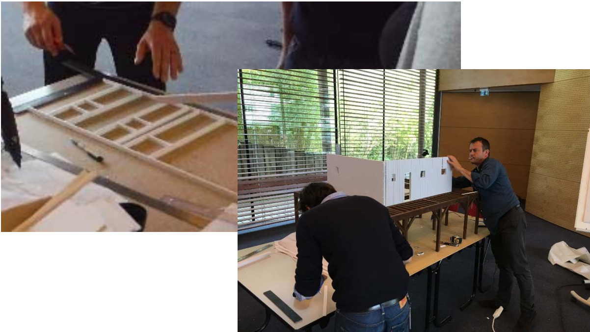
Figure 20: jig to speed up the fabrication process
