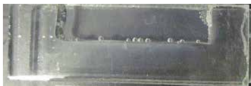
FIG. 4 Transparent Structural Sealant after 10000 hours UVA exposure
