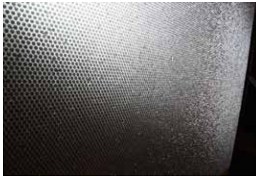
FIG. 7 BlingCrete – Light reflecting concrete, R&D: BAU KUNST ERFINDEN // BUILDING ART INVENTION, University of Kassel, T. Klooster, R. Polster, J. Juraschek, M. Hellmann, F. Ecke and H. Klussmann, funded by the BMWi/ ZIM, Photo: BAU KUNST ERFINDEN
