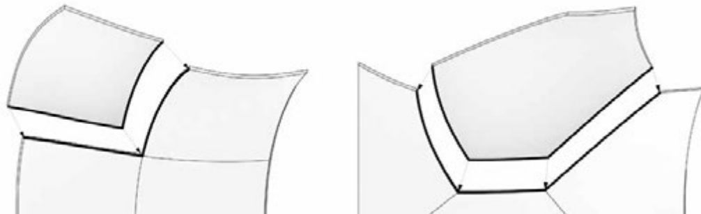
FIG. 8 Segmentation dependent edge assembly (left | quadrangular Segmentation, right | hexagonal Segmentation)
