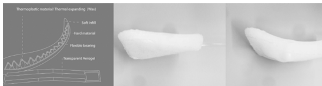
FIG. 11 Left: Section of volume chamber, Middle and Right: Model with integrated volume chamber to specify the movement with a thermodynamic material
