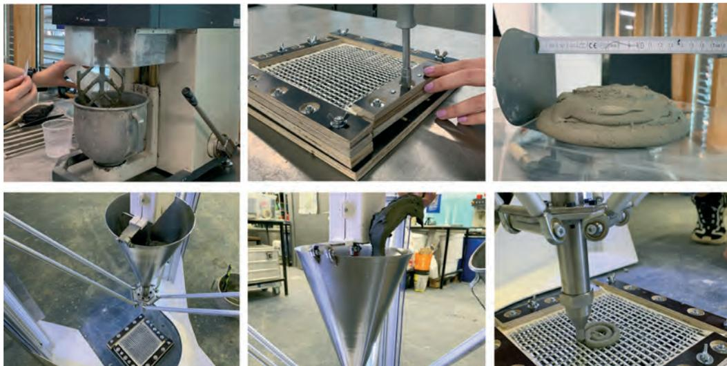
FIG. 16 3D printing process from top left to bottom right: Textile attachment, concrete mix, breakout test, 3D printer preparation, printer hopper filling, 3D printing on spacer textile made of AR glass © FRAUAS
