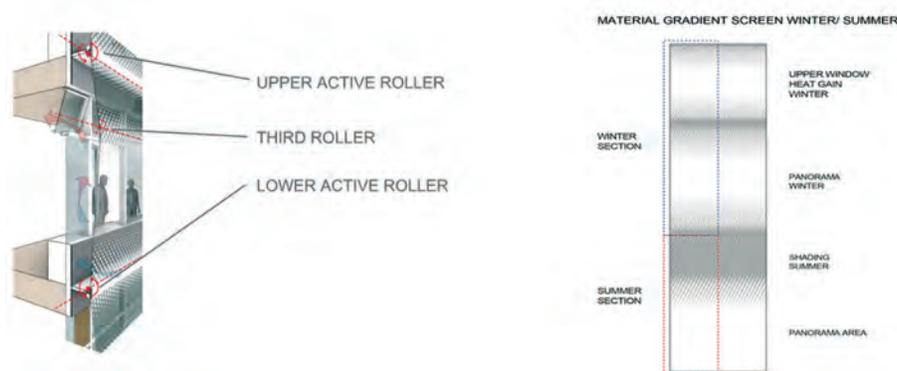
FIG. 7 Roller configuration (l.) for intended material gradient (r.)
