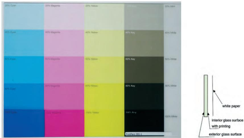
FIG. 9 4mm low iron glass printed in semi-transparent CMYK-White colours with increasing saturation from top to bottom as colour sample placed in front of a glossy white paper as reflecting surface.
