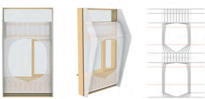
FIG. 19 Section perspective illustrating a typical office environment relative to the screen façade. Combined textile and membrane screen (in progress)
