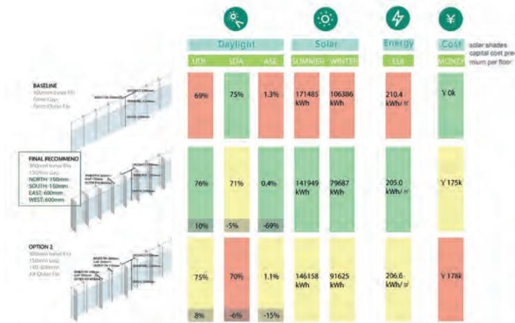
FIG. 10 View of the interface of the summary report module of the External Fins Optioneering case.
