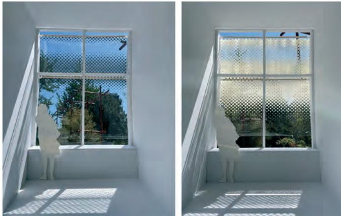
FIG. 18 Photograph of model taken outdoors with the winter screen (left) and the summer screen (right)
