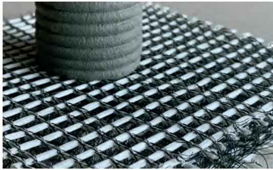
FIG. 17 3D printing with concrete on a chain-knitted biaxial spacer fabric made of AR glass with knitted and pile threads from PES © FRAUAS
