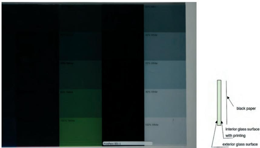
FIG. 10 4mm low iron glass printed semi-transparent CMYK-White colours with increasing saturation from top to bottom as colour sample placed in front of a glossy black paper as reflecting surface.
