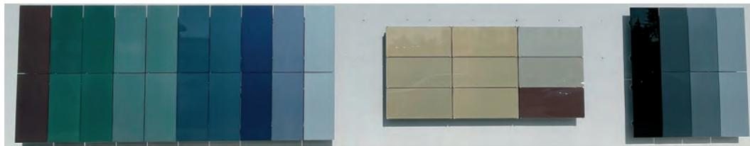
FIG. 24 Colour sample using transparent effect pigments.
