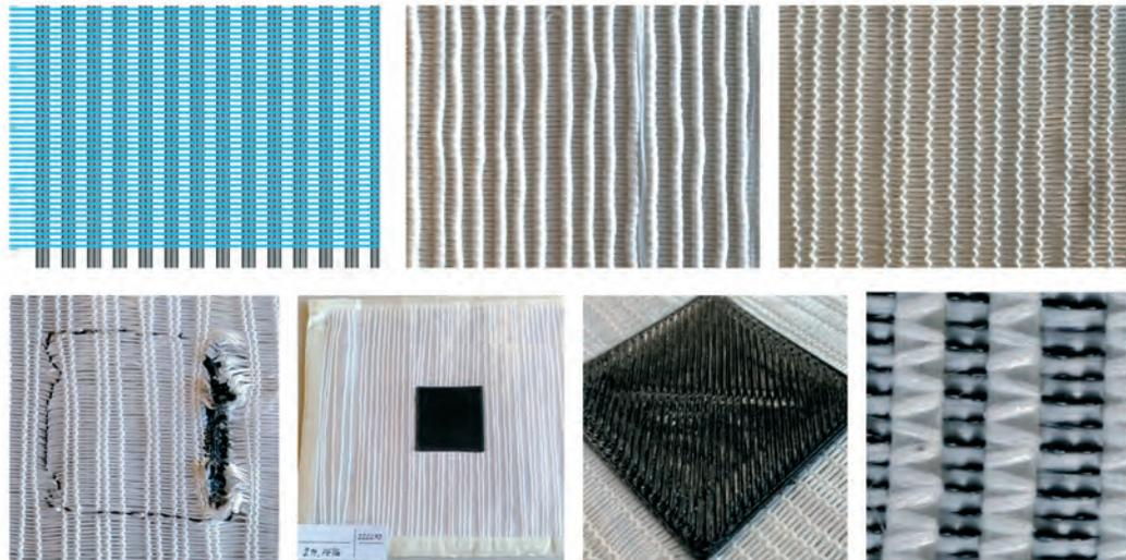
FIG. 9 Top left: Design of a biaxial warp-knitted fabric based on theoretically determined roving cross sections; top centre: Bottom view of the produced textile; top right: Top view; bottom left: 3D printing with rPETG on iaxial warp-knitted fabric; bottom centre: Print parameter optimisation – Z-offset and infill; bottom right: Close up, bottom view – textile with visible print material penetration © FRAUAS
