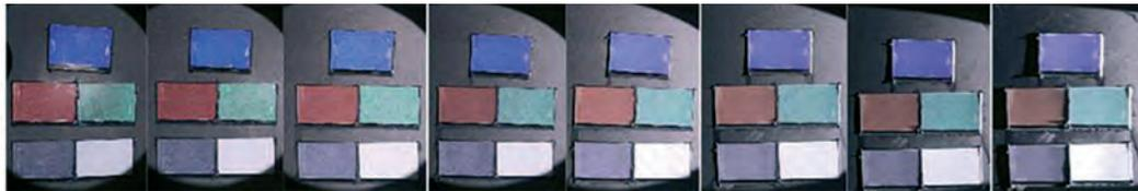
FIG. 20 Series of photographs of colour sample blue, red, green, dark grey, light grey taken with 8 different angles of direct irradiation (10° left to 80° right) while the angle of perception is kept constant perpendicular to the plane of the module.
