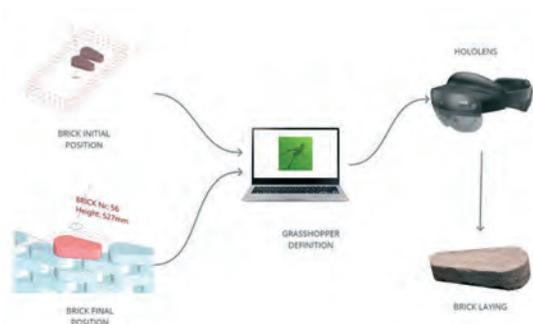
FIG. 2 Assembly procedure, from parametric design to bricklaying
