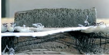
FIG. 15 Side view of spacer warp-knitted non-crimp textile with the distribution of the concrete © FRAUAS
