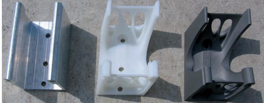
FIG. 1 From standard aluminium extrusion (left) to ABS prototype (middle) to 3D printed stainless steel connector (right)
