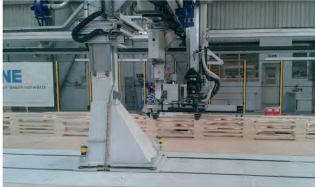
FIG. 7 Erne AG, gantry robot assembling a 3D roof truss
