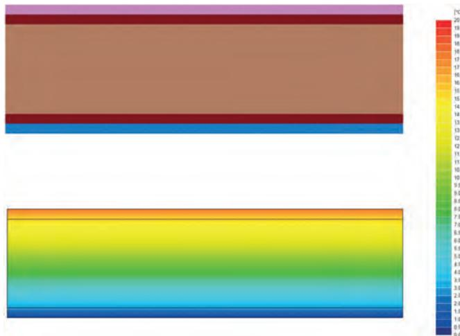
FIG. 8 Build-up and isothermal lines for Case 1, horizontal section
