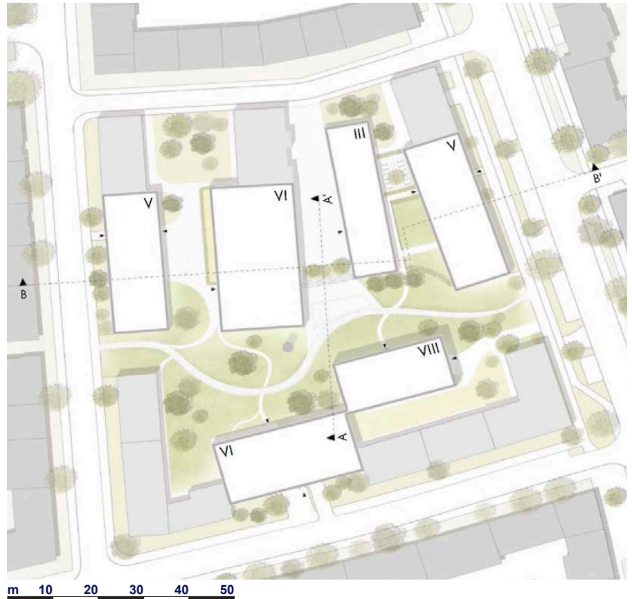
Site plan. The linear open zones, oriented north-south, support various functions, including a central work zone accessed from the north. The distribution of uses supports the co-existence of housing, community-oriented uses, and production.
