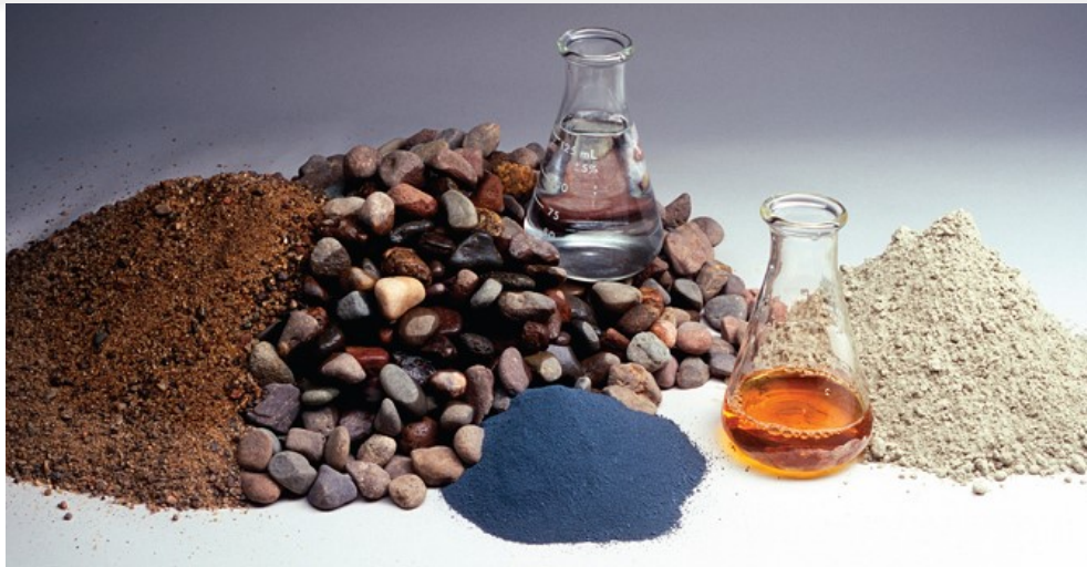
Components for the concrete mix
