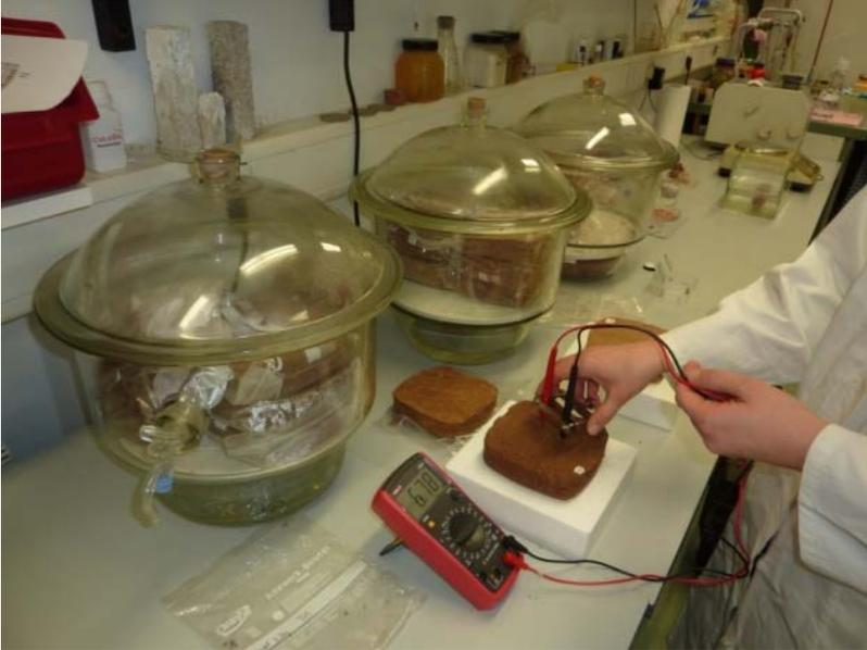
Figure 7: test measuring on artificial specimens using UT601-2 in the ProDenkmal lab. The conditioned test specimens were packed in plastic foils and stored in conditioned glass desiccators.
