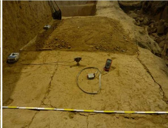
Figure 21: Finished removing of the poultice around the sentec probe P1 (arrow).
