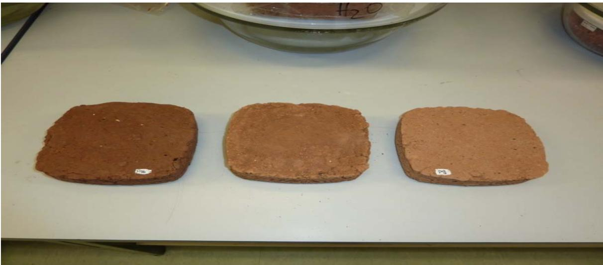
Figure : Test specimens of different moisture. Test specimen size: 13cm:13cm:6cm
