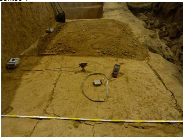
Fig. 12: Finished removing of the poultice around probe 1. Probe 2 remains covered by dried out poultice and plastic foil.
