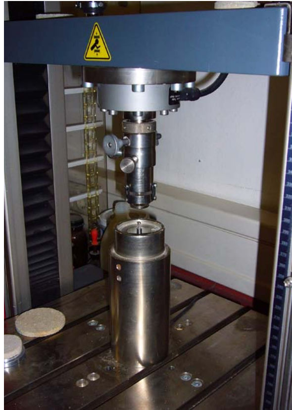
Fig. 38: Test set-up to measure biaxial flexural strength
