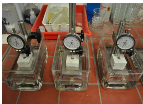
Fig. 30: Measuring set-up to determine hygric dilatation
