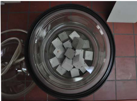
Fig. 23: Samples in the dessicator after flooding with water
