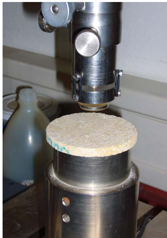
Fig. 39-41: Two column Universal testing machine and test set-up to measure biaxial flexural strength
