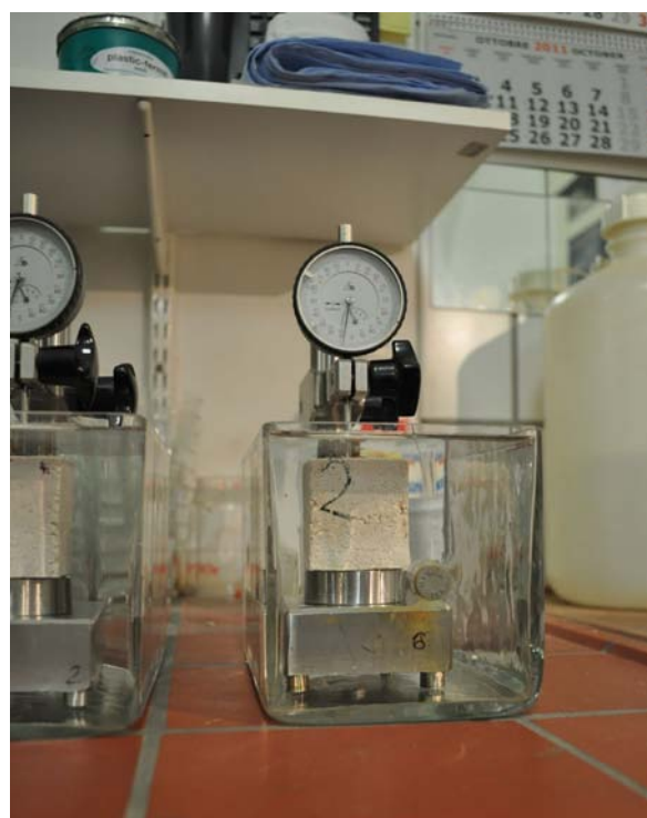
Fig. 32: Measuring set-up to determine hygric dilatation
