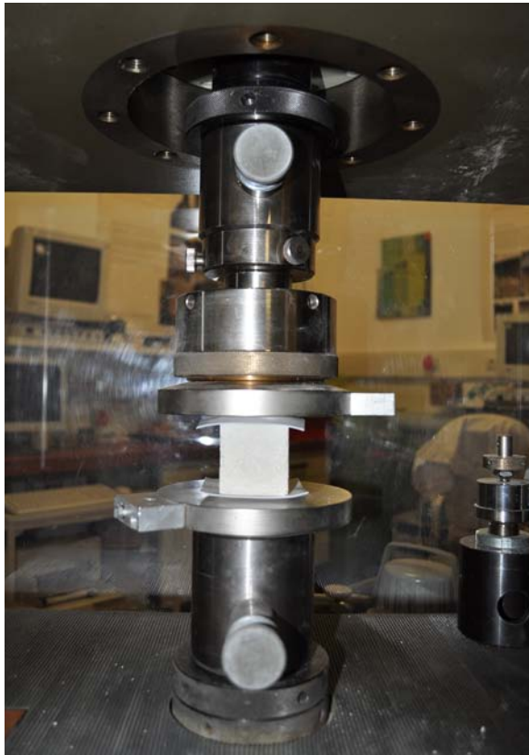
Fig. 43: Compression strength test on one of the cubes of the stone consolidation materials
