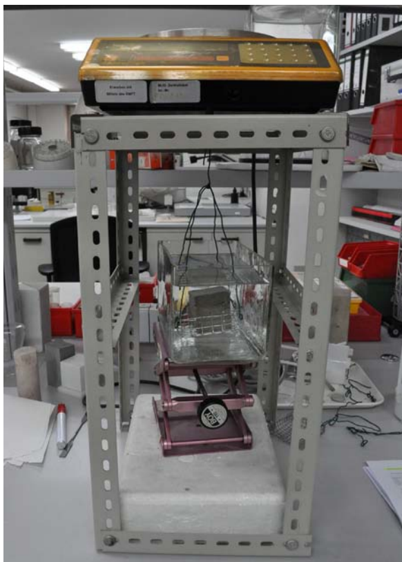
Fig. 25-28: Measuring set-up to determine the mass of a body under water (Archimedes' principle, the weight and buoyancy of the weighing basket are taken into account in the calculation)
