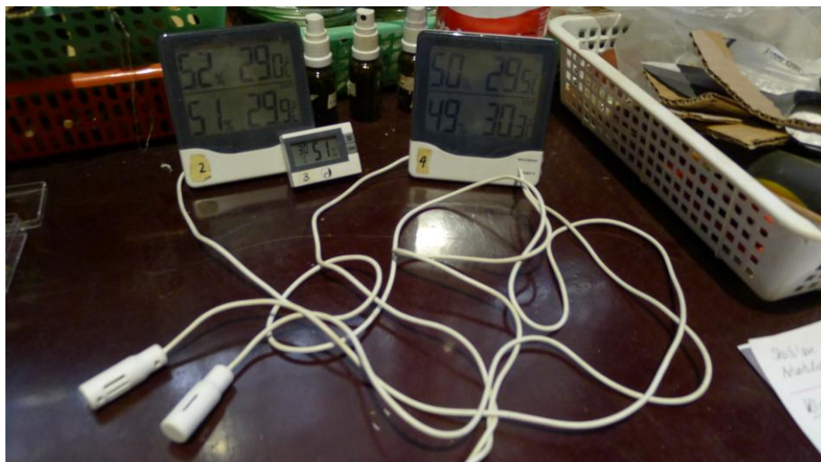
Fig. 116 The three hygrothermometers with differing measuring data, even if positioned next to each other.
