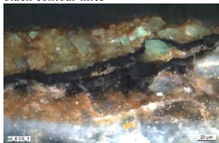
Fig. 433: sd 8 CS 1: ground layer stained brown; paint layer and two black contour lines
