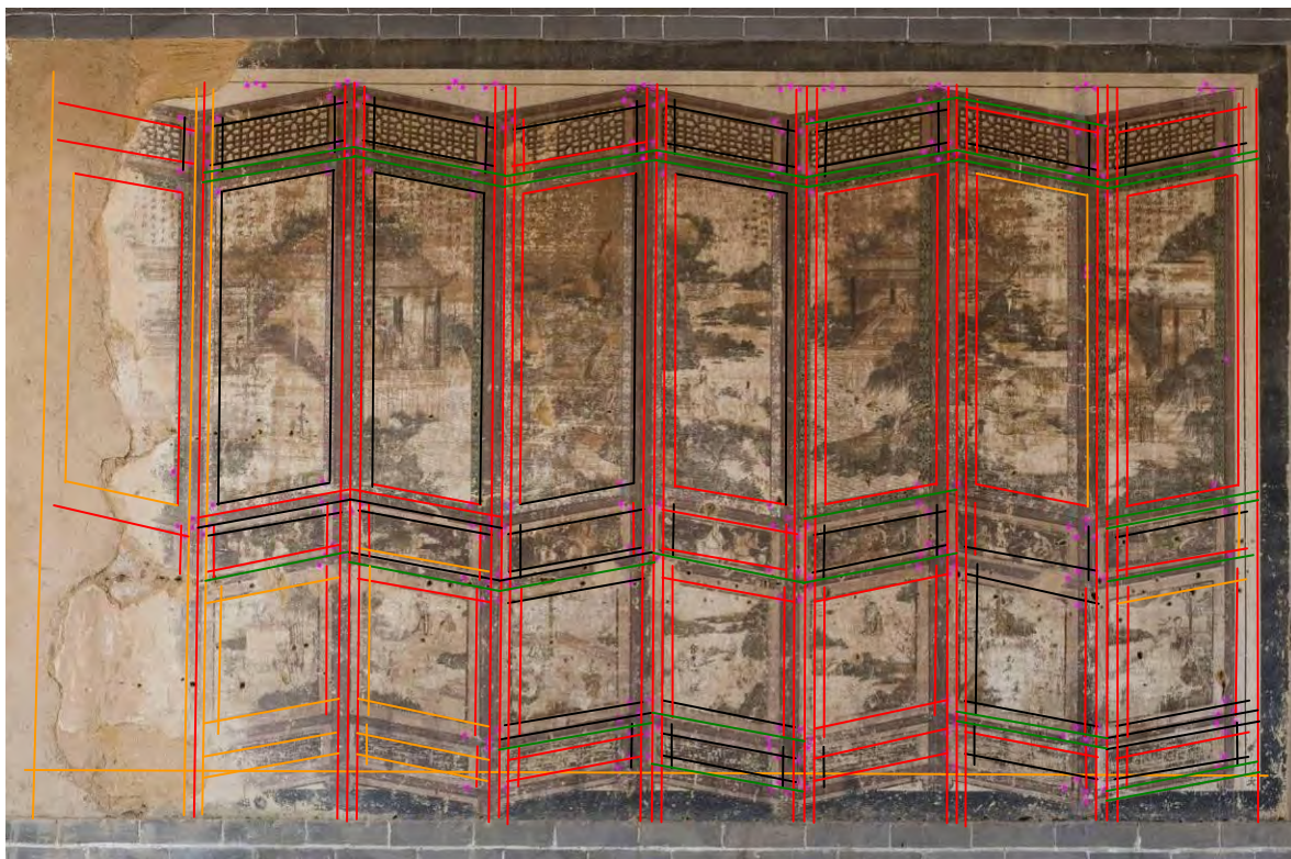
Fig. 92 Reconstruction of strings used for the construction of the folding screen, (photograph not rectified) [Photograph: Shaanxi Institute for Conservation]
