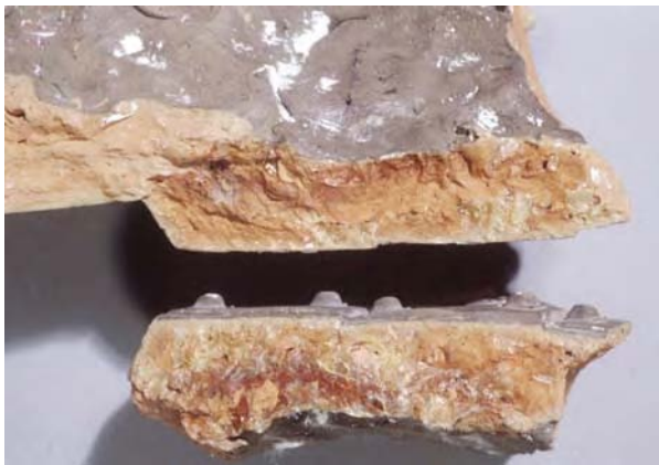
Fragments U 6 and U 7, glued with epoxy resin and a primer, after opening the joint again.
