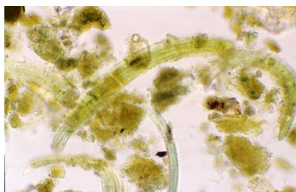
Fig. 5. B-002/02, prep. no. 15, transmitted polarised light, 100x magnified: Malachite in various shapes including "banana"-shaped fibrous particles
