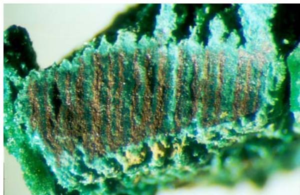
Fig.1. B-001/02: particle with visible layer structure (red and green) on the fracture edge, 8.0x magnified
