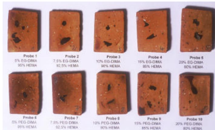
Original lacquer consolidated on modern terracotta slabs, treated with acrylate formulation (see description below the slabs) and irradiated (electron beam, 1MeV, 2mA, 60 kGy)
