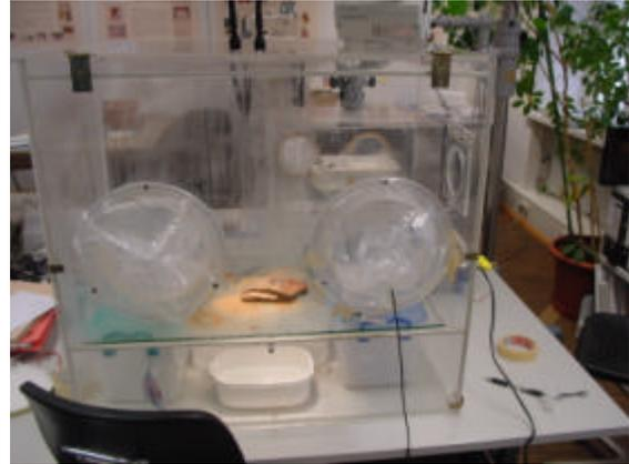
Fig. 8. Perspex box during cleaning of F-008/03. The set-up inside the box is visible. For illumination, a "cold light" lamp was placed on top of the box. The air brush is introduced through the right arm hole of the front flap.
