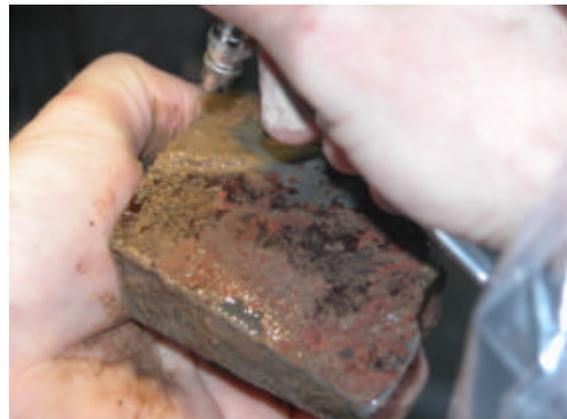
Fig. 10. Detail of the cleaning of the painted surface of F-008/03.
