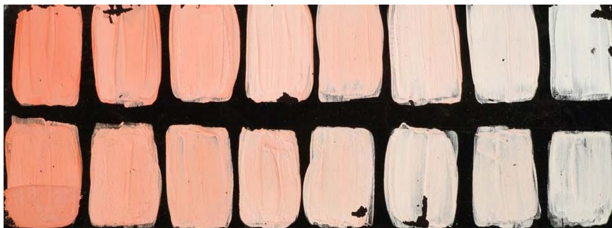
Fig. 30. Sequence of mixtures for flesh tones with zhusha and two different mixtures of white: top row: lead white /bone ash 1:1; lower row: bone ash
