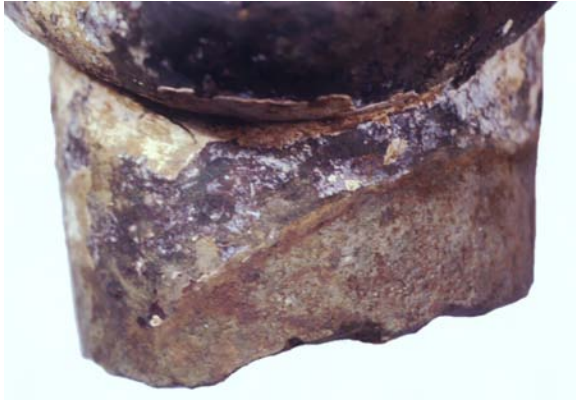
Fig. 9: Head/2002 – priming barb at the throat following the line of the collar
