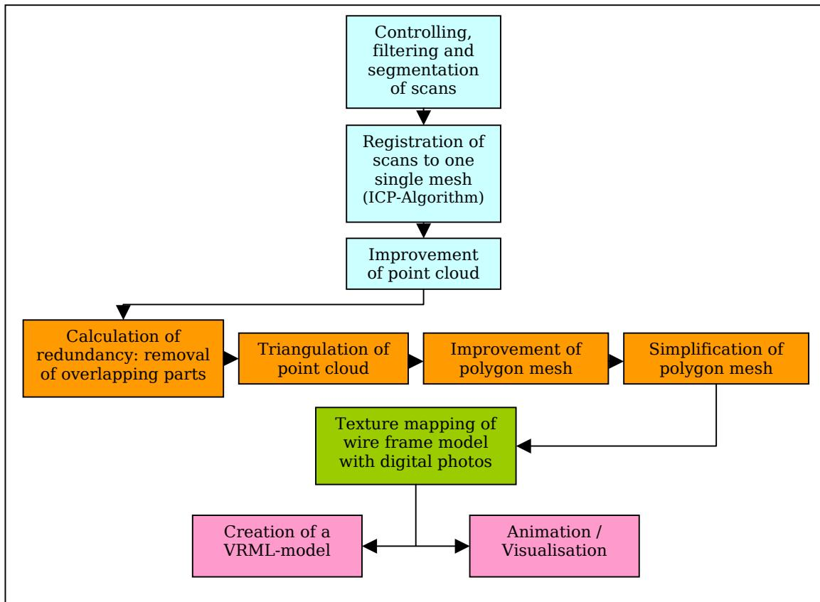
**Figure 3:** Schematically workflow (diagram by ArcTron GmbH).
