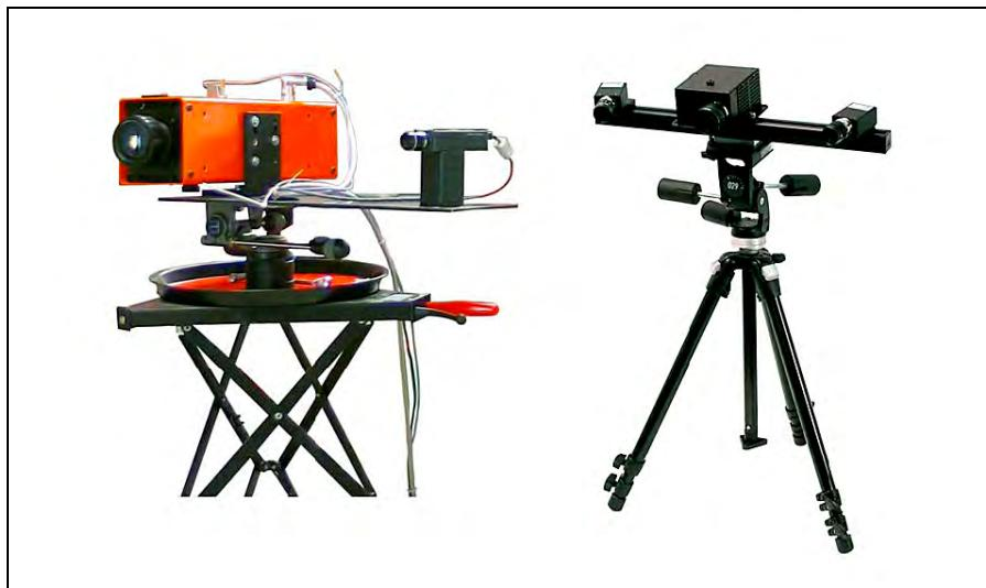
**Figure 1:** The two QT Sculptor measuring systems (two different types, right: QT Sculptor P-TM 1024).
