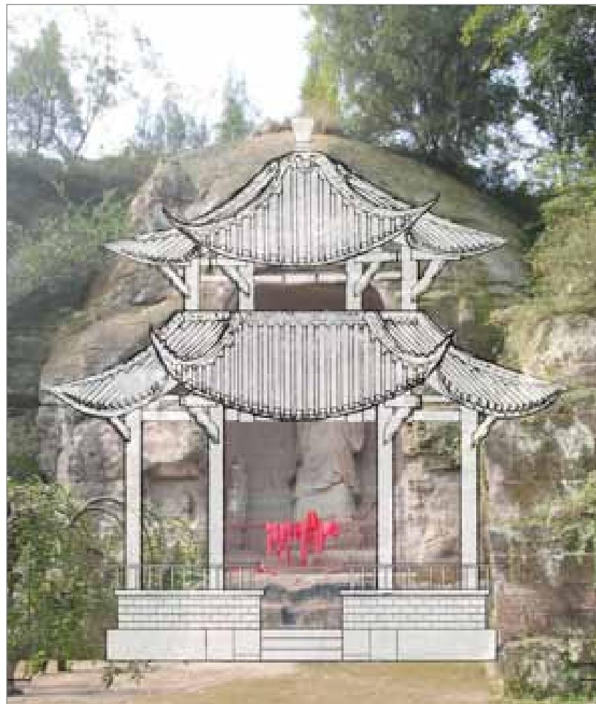
**Fig. 9:** Elevation of the planned pavilion in front of niche no. 10
