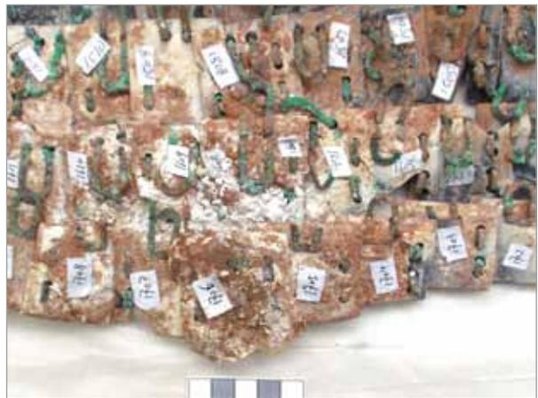
Fig. 4 | Burnt plates at the lower end of BB1
