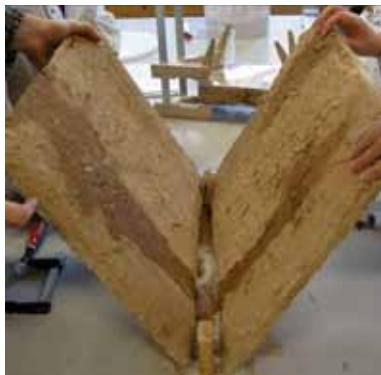
Moistening of the clay walls with water. Front and backside of the void was sprinkled with a prepared cannula
