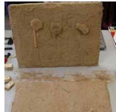
The mortars have formed a stamp in the hollow. Good fixing after drying on front- and backside
