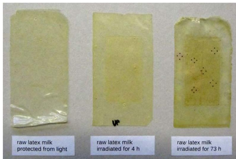
Figure B.2: Cast films of natural latex milk, new and artificially aged for 4 and 73 hours.
