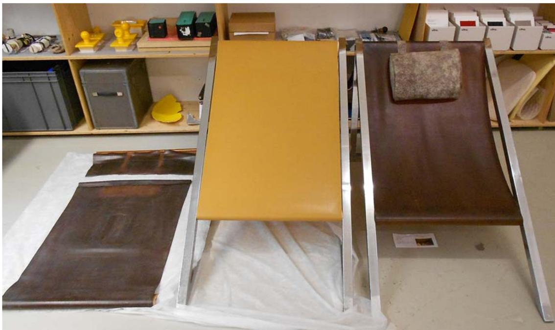
Figure 5.2: Original and replacement seating of the chaise longue “Mies” by ARCHIZOOM in the conservation studio of the Vitra Design Museum in 2011. Left: dismounted darkened and torn original seat cover from 1969. Centre: chaise longue with new seat cover. Right: chaise longue with oxidised, darkened and stripped out seat cover.
