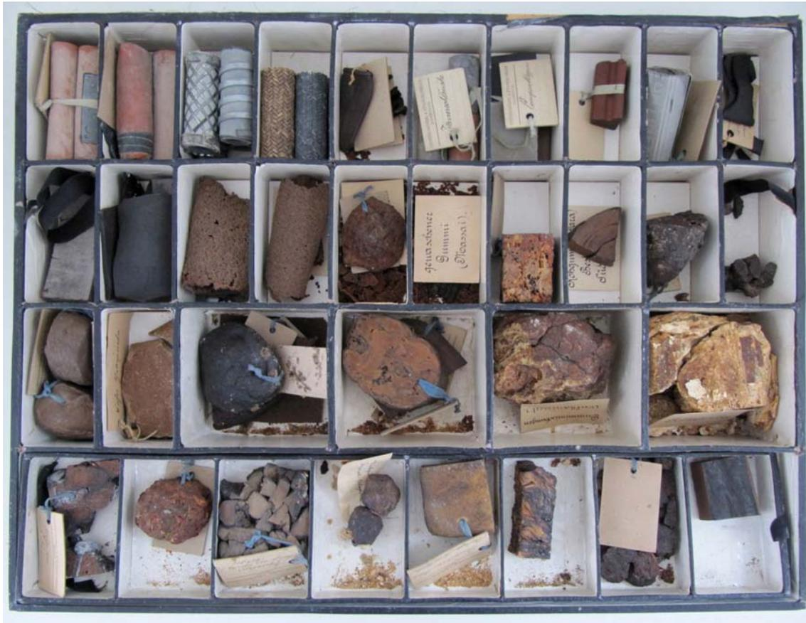
Figure 5.1: Sample case with naturally degraded, uncompounded and unvulcanised rubber materials (hevea and gutta type) from different continents as well as few vulcanised product samples.
