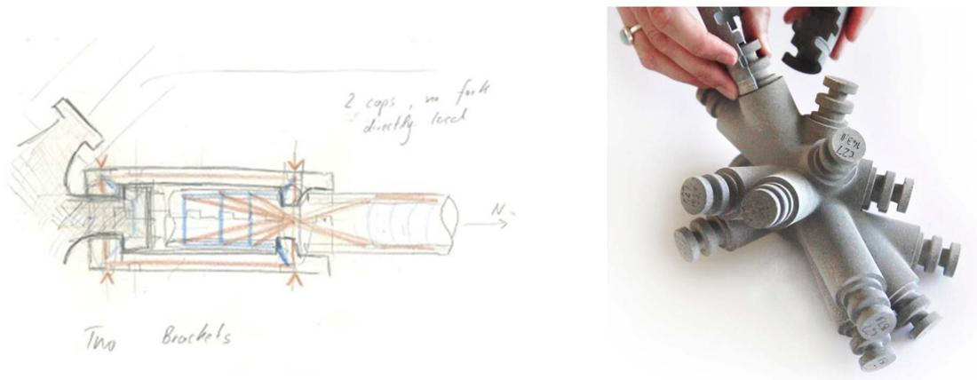
Figure 9: Equilibrium-based methods provided the basis for developing a connection that fulfilled the mechanical requirements and ensures the required hinge behavior and assembly tolerance. [Photo: A. Bargetzi]
