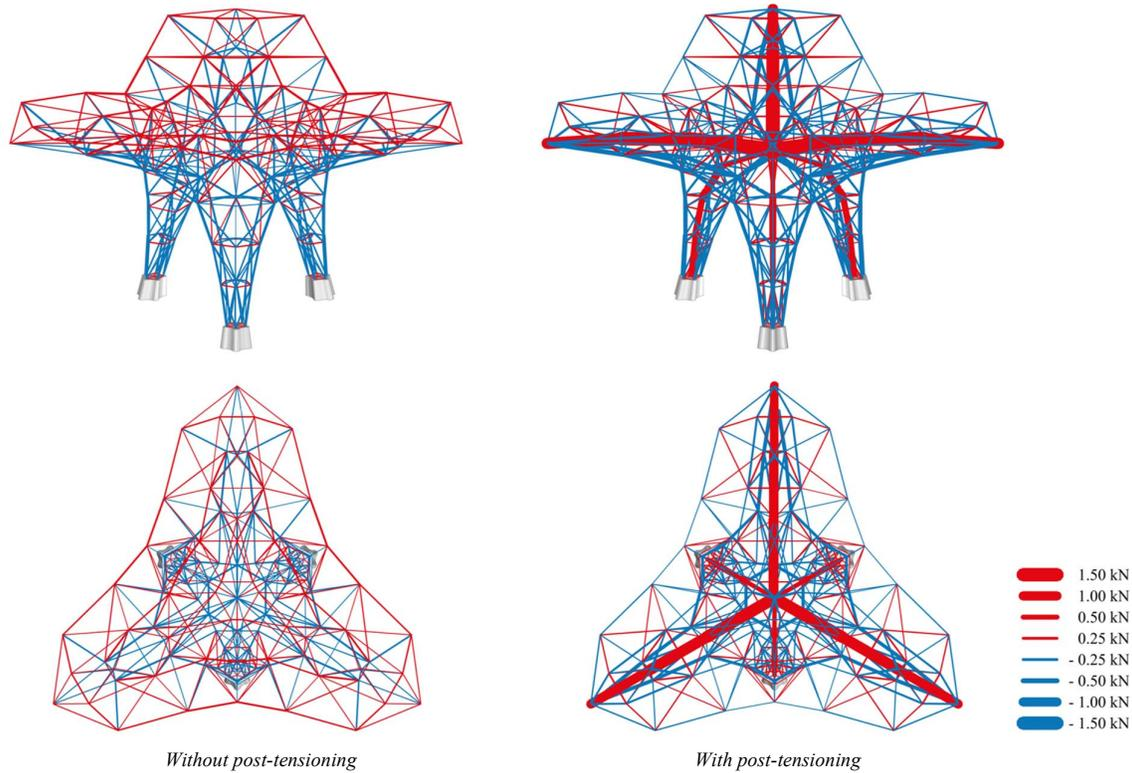
Figure 11: Structural analysis (axial forces) of the Digital Bamboo without and with post-tensioning cables. Using post-tensioning allows significantly reducing the number of bamboo canes under tension.
