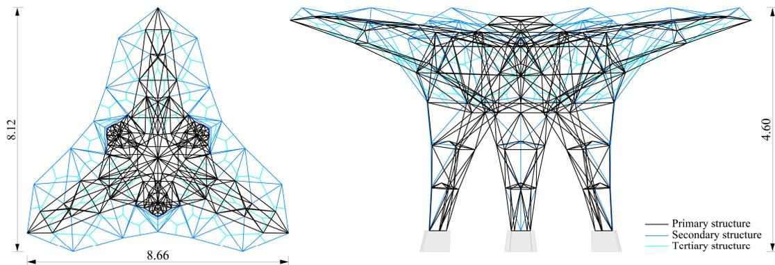
Figure 4: The hierarchical space frame structure of Digital Bamboo is composed of primary, secondary and tertiary sub-structures.
