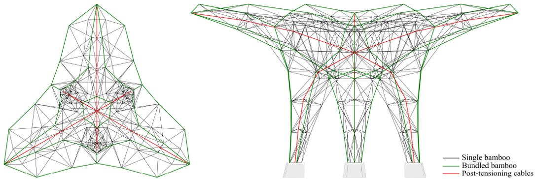
Figure 8: Schematic representation of the bundled elements and the six post-tensioning cables.
