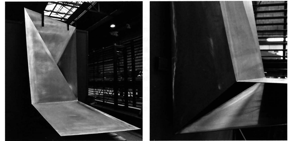
Fig. 6 Fabrication of final design out of folded steel plates of 3mm thickness
